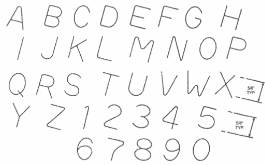
Figure 4-2-2. Design of Special Letters and Numbers on a 10 Degree Angle for Rail Stamps, No Sharp Corners
